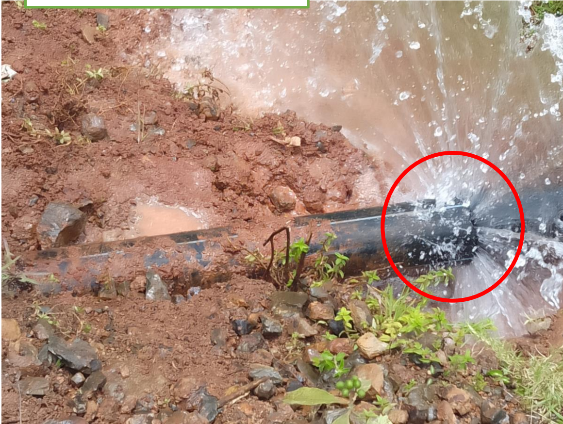
Failed Butt Fusion Joint
